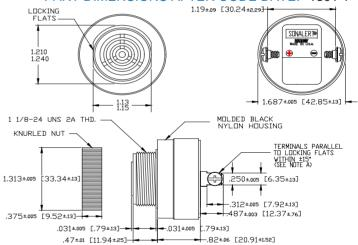
NOTE A: TERMINALS-.032 BRASS TIN PLATED, TAPPED FOR #6-32 SCREW, TVOI #6-32 NICKEL PLATED BRASS SCREWS INCLUDED, WILL ACCEPT 1/4' QUICK CINNECT. NOTE B: MOUNTING- REMOVE BLACK PLASTIC NUT AND INSERT THREADED FRONT THROUGH 1.25' HOLE PUNCHED IN PANEL, IF ORIENTATION IS NEEDED, NOTE LOCKING FLATS ON DRAWING, SCREW NUT BACK UN. DO NOT OVERTIGHTEN.
