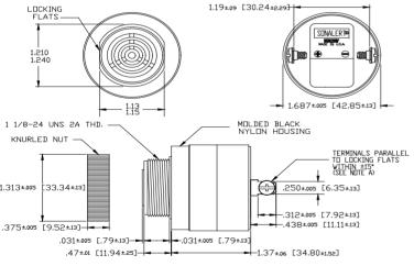
NOTE A: TERMINALS-.032 BRASS TIN PLATED, TAPPED FOR #6-32 SCREW, TWD #6-32 NICKEL PLATED BRASS SCREWS INCLUDED, WILL ACCEPT 1/4' QUICK CONNECT. NOTE B: MOUNTING- REMOVE BLACK PLASTIC NUT
