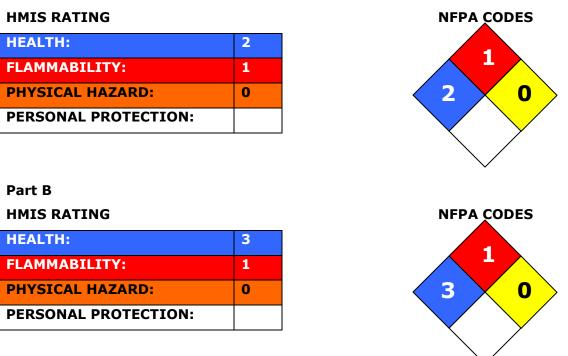
Health and Safety: The 8321C parts can ignite if the liquid is heated and exposed to flames or sparks.
