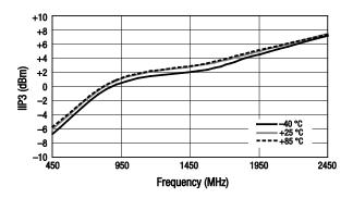
Figure 5. IIP3 Over Temperature and Frequency
