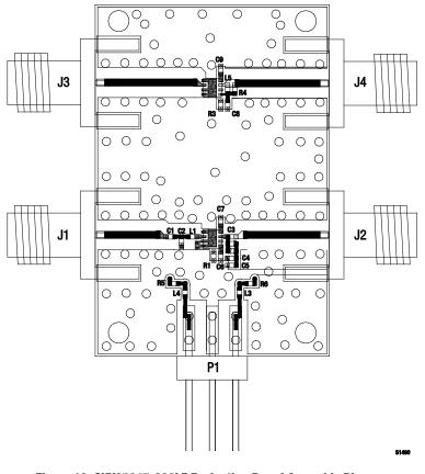
Figure 12. SKY65047-360LF Evaluation Board Assembly Diagram (1575 MHz)
