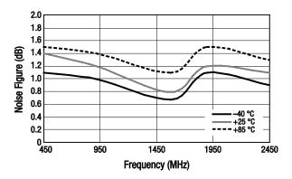
Figure 7. Noise Figure Over Temperature and Frequency
