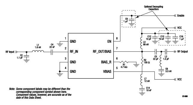
Figure 13. SKY65047-360LF Evaluation Board Schematic (2450 MHz)
