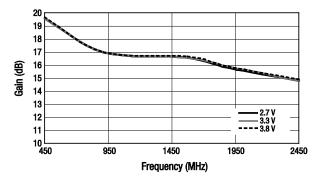
**Figure 4. Gain Over Supply Voltage and Frequency**
