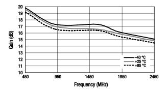
Figure 3. Gain Over Temperature and Frequency
