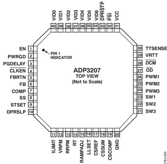
Figure 5. Pin Configuration
