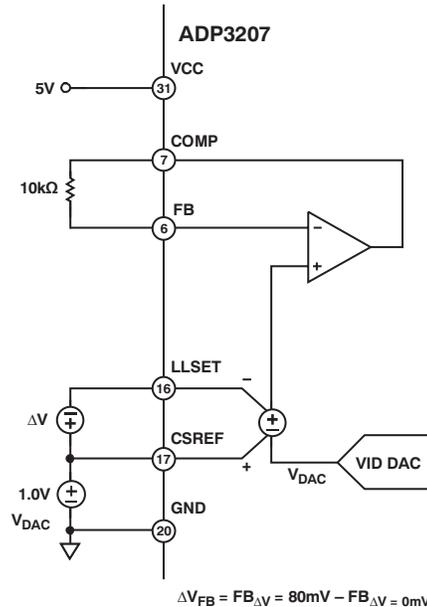
Figure 4. Positioning Accuracy
