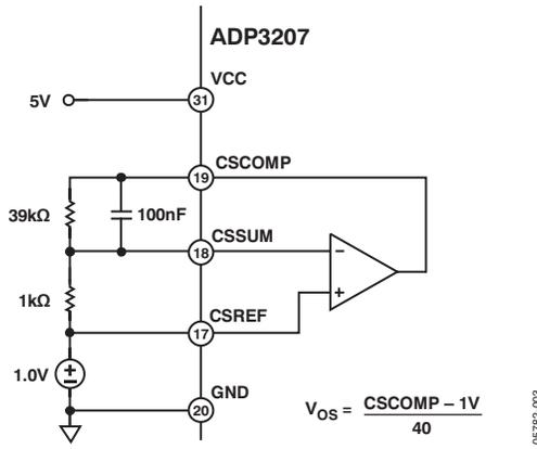
Figure 3. Current-Sense Amplifier  $V_{os}$
