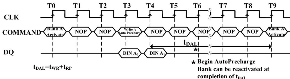
**Figure 14. Burst Write with Auto-Precharge (Burst Length = 2)**
