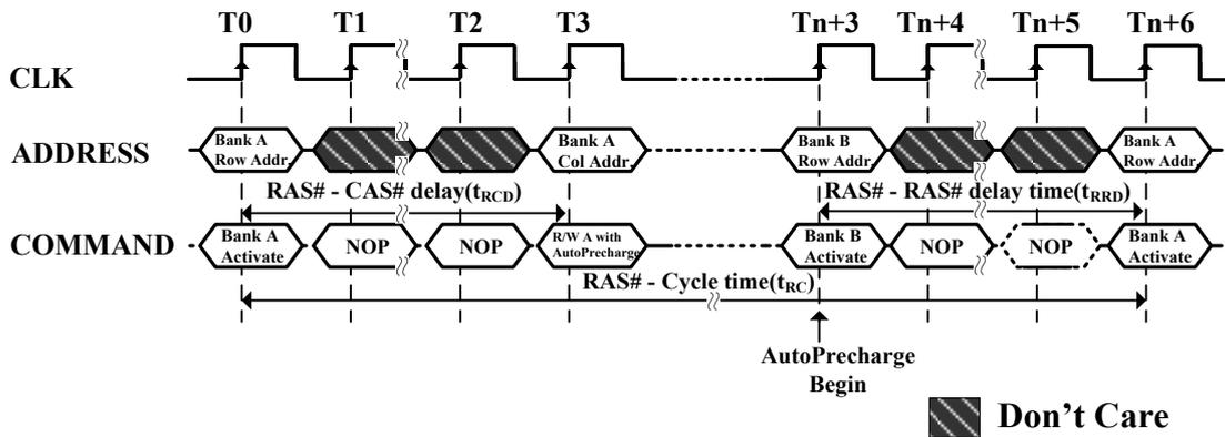
**Figure 3. BankActivate Command Cycle (Burst Length = n)**
