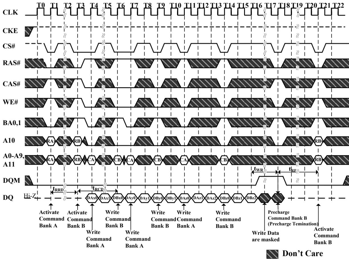
Figure 42. Precharge Termination of a Burst
