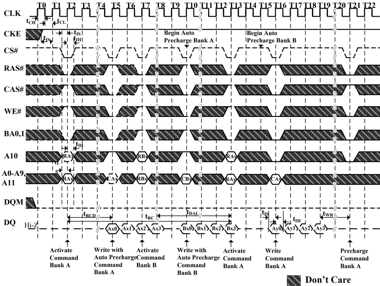
**Figure 20. AC Parameters for Read Timing (Burst Length=2, CAS# Latency=2)**
