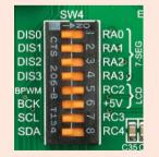
IMPORTANT: In order to use PWM back-light both SW4.5 and SW4.6 switches must be enabled at the same time.
