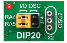
Figure 4-8: RA4 and RA5 as I/O pins (when using internal oscillator)
