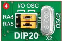
Figure 4-9: RA4 and RA5 connected to X2 quartz-crystal
