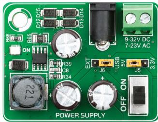
Figure 3-1: Dual power supply unit of EasyPIC™ v7
