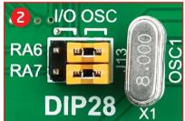
Figure 4-7: RA6 and RA7 connected to X1 quartz-crystal
