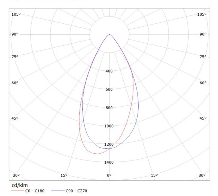
Luminaire: Ledil Oy CA11022\_TINA2-W (Nichia NVS19 98lm @ 250mA) Efficiency=82% Lamps: 1 x Nichia NVS19 98lm @ 250mA
