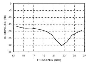
**Output Return Loss vs. Frequency**
