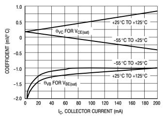
**Figure 18. Temperature Coefficients**
