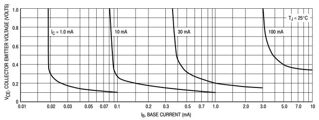
Figure 16. Collector Saturation Region
