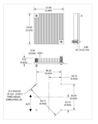
Width: 57.90 Length: 59.00 Height: 11.00 Base Thickness: 2.80 Fin Thickness: Length , Width 0.50 # of Fins: Length , Width 18 Fin Tip to Tip: Finish: AavSHIELD 3C
