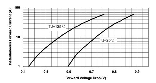
Fig.3-Typical Instantaneous Forward Voltage Characteristics
