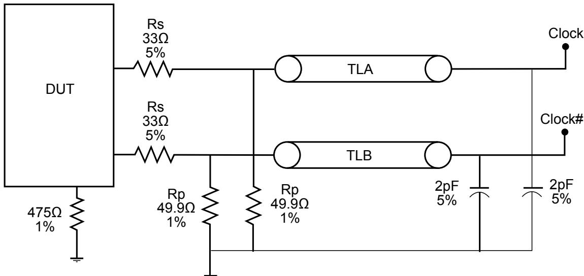
**Configuration Test Load Board Termination for LVPECL/ LVDS Outputs**
