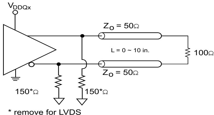
**Configuration Test Load Board Termination for LVC MOS Outputs**
