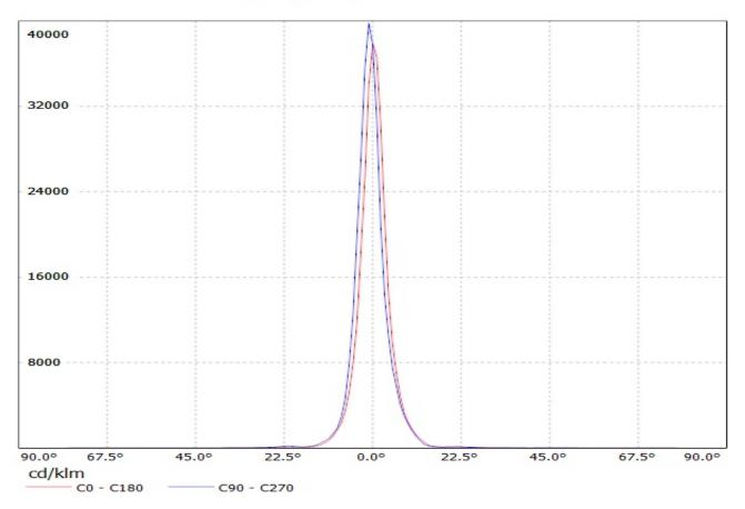
Luminaire: Ledil Oy CP12412\_LOS-RS\_(Osram\_Oslon\_Square\_EC)\_SIMULATED Lamps: 1 x Osram Oslon Square GW CSSRM1.EC
