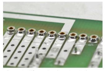
Part number MS11 consists of a carrier strip of 30 cage jacks. The strip can easily be cut to any desired number of cage jacks. These are mounted directly in a print circuit board. After soldering, the carrier is pulled off the cage jacks. Use a spacer between the PCB and the heatsink to avoid short circuits.
