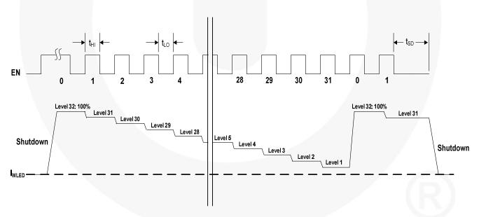
Figure 14. Digital Pulse-Dimming Control Diagram
