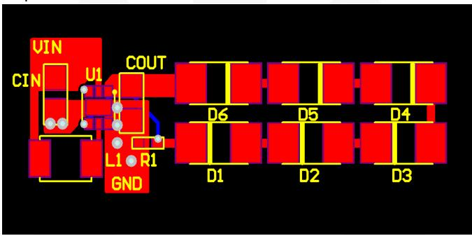
Figure 15. Recommended Component Placement
