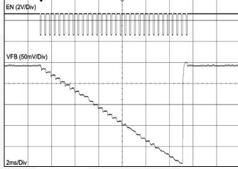
Figure 10. Line Transient Response for 6 LEDs
