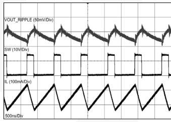
Figure 13. Steady-State Waveform for  $V_{\text{OUT}}$ , Switch Voltage, and Inductor Current for 6 LEDs
