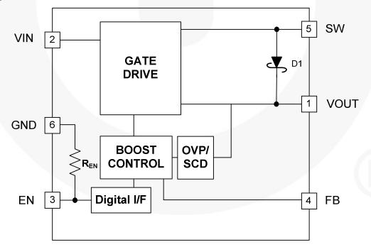
Figure 2. Block Diagram
