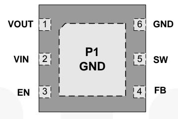
Figure 3. UMLP6 Package (Top View)
