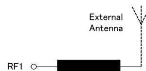
Figure 7: One external antenna
