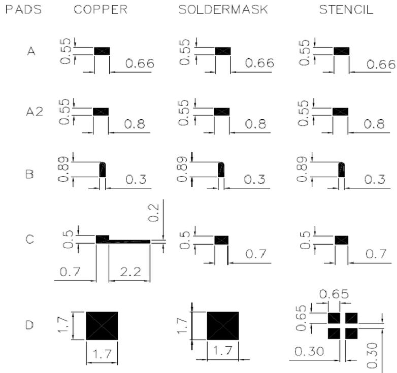
Figure 19: Copper pad, solder mask opening and stencil
