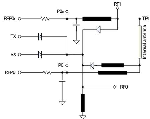
Figure 6: Internal circuit of the SC14WAMDECT SF
