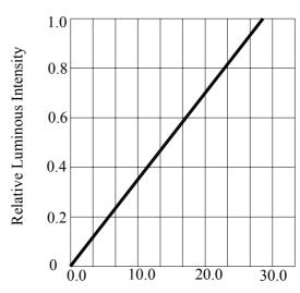
FORWARD CURRENT VS. LUMINOUS INTENSITY
