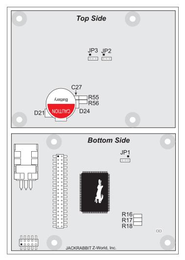
Figure A-2. Location of BL1810 Configurable Positions
