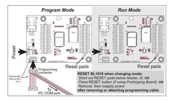
Figure 5. BL1810 Program Mode and Run Mode Setup
