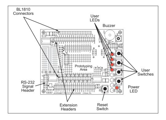
Figure 1. Prototyping Board
