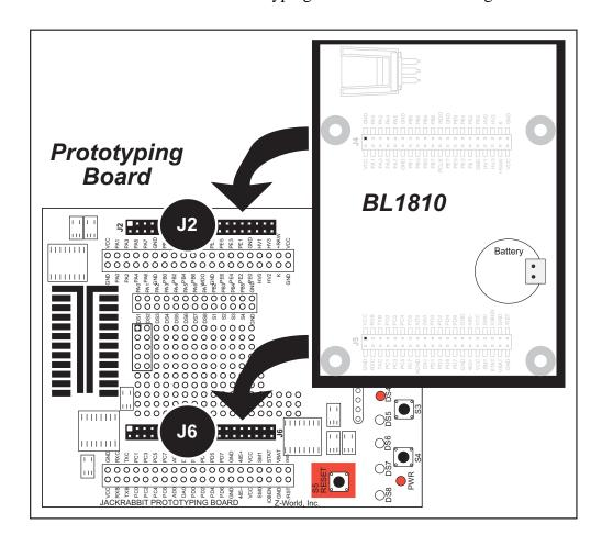
Figure 2. Attach BL1810 to Prototyping Board
