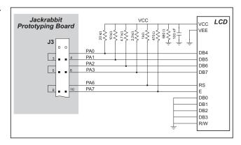
This sample program only involves writing, and that is why we ground the R/W pin. VEE is used to control brightness—the simplest thing to do is ground it. If you need to control the brightness, you can connect a potentiometer between ground and -5 V, with the arm going to the VEE pin. Check the specs on the LCD before doing this as some LCDs may require a different connection. VCC is +5 V and VSS is ground.
