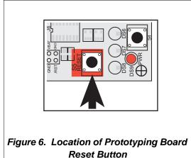
2. Reset the BL1810. You may do this as explained in Figure 5. Figure 6 shows the location of the RESET button on the Prototyping Board.
