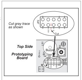
Figure 7. Cut Trace on Prototyping Board When Vcc and K Are Different
