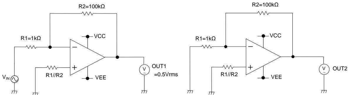
Figure 27. Test Circuit 3(Channel Separation)
