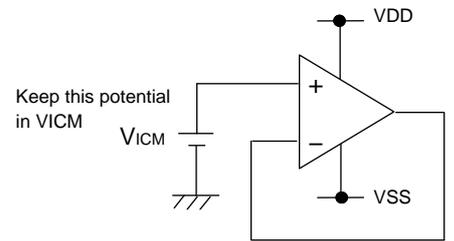
Figure 33. Example of Application Circuit for Unused Op-amp
