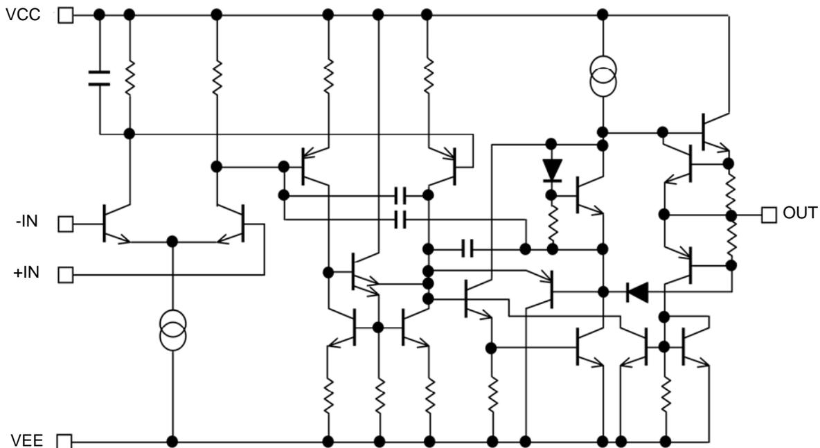
Figure 1. Simplified Schematic (1channel only)
