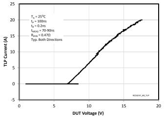
ESD Clamping (-8kV Contact per IEC 61000-4-2)
