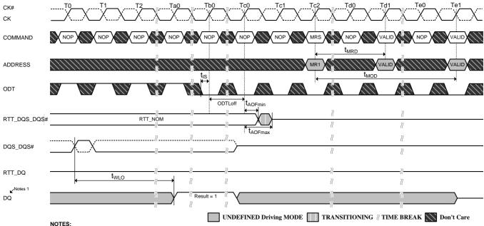
1. The DQ result = 1 between Ta0 and Tc0 is a result of the DQS, DQS# signals capturing CK high just after the T0 state.
