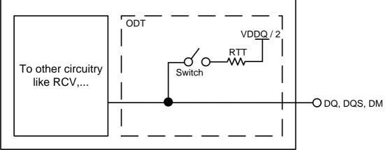
The switch is enabled by the internal ODT control logic, which uses the external ODT pin and other control information. The value of RTT is determined by the settings of Mode Register bits. The ODT pin will be ignored if the Mode Register MR1 and MR2 are programmed to disable ODT and in self-refresh mode.
