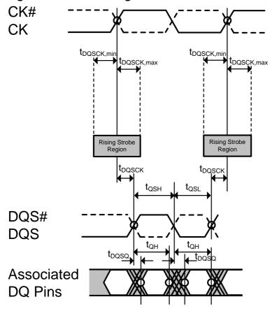
Figure 18. READ timing Definition
