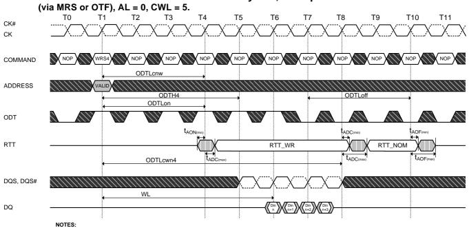
1. ODTH4 is defined from ODT registered high to ODT registered low, so in this example, ODTH4 is satisfied. TRANSITIONING DON'T CARE 2. ODT registered low at T5 would also be legal.
