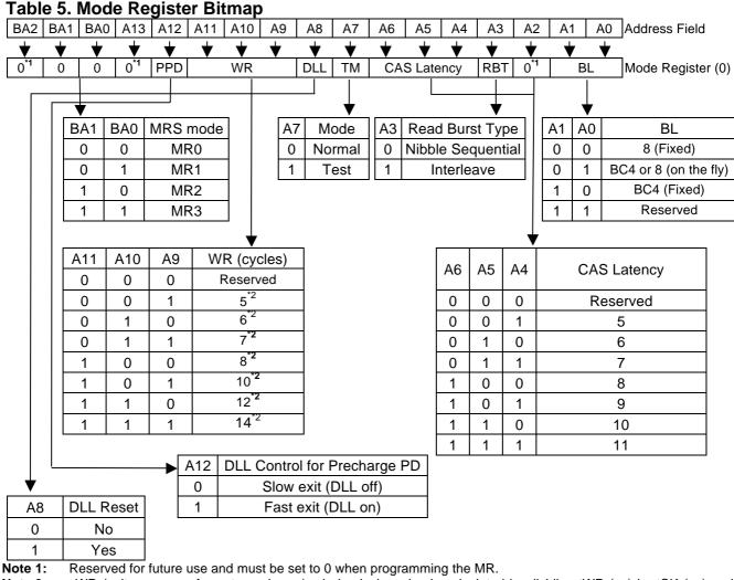
**Note 2:** WR (write recovery for autoprecharge) min in clock cycles is calculated by dividing tWR (ns) by tCK (ns) and rounding up to the next integer WRmin [cycles] =Roundup (tWR / tCK). The value in the mode register must be programmed to be equal or larger than WRmin. The programmed WR value is used with tRP to determine tDAL.
