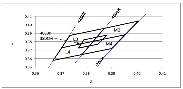
Figure 13: Graph of Neutral White Test Bins in xy Color Space
