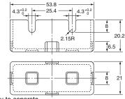
Note: The Cover has six thin, easy-to-separate portions for easy lead wire connections.
