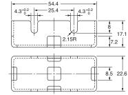
Note: 1. The Cover has five holes for easy lead wire connections. 2. AP1-A should be used with the AP-A
