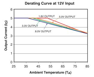
Thermal de-rating curves for DFN-8 package part under typical input and output conditions. Circuit of Figure 1. 25°C ambient temperature and natural convection (air speed < 50LFM) unless otherwise specified.
