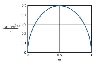
Figure 2. I<sub>CIN</sub> vs. Voltage Conversion Ratio
