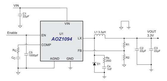
Figure 1. 3.3V/5A Buck Down Regulator
