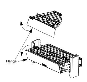
The hinged cover opens from the top or the bottom. Pull flange to open and close cover.
