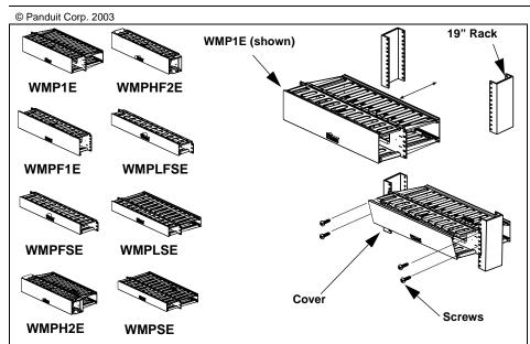
Install the managers to the rack with the #12-24x.5 or M6 screws provided. Built-in screw retention in mounting holes secures screws in manager during installation. Install the covers to the manager by positioning cover flat against the front of the manager fingers, then push to snap in place.
