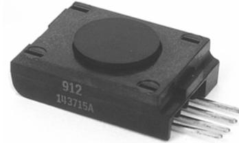
The FS01/FS03 sensors are special low cost, peizoresistive-based force sensors. These high-level voltage output, calibrated, and temperature compensated sensors give an accurate and stable output over a 5 °C to 50 °C [41 °F to 122 °F] temperature range. They offer simple operation from a single 5.0 Vdc supply. Operation from any DC supply voltage, up to 12.0 Vdc, is acceptable.
