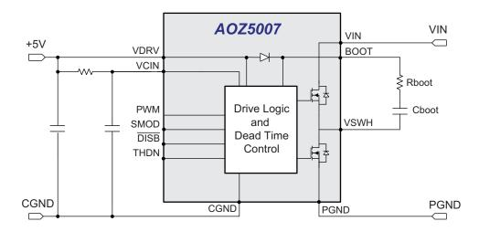
Figure 17. Applying VDRV and Generating BOOT Supply
