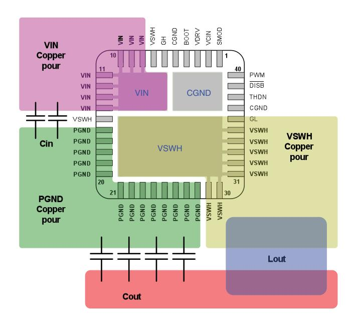
Figure 18. PCB Layout Illustration for Minimizing Current Loops
