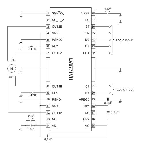
Each constant setting formula of above circuit example is as below. Setting of chopping frequency: 31kHz (FC = Low)
