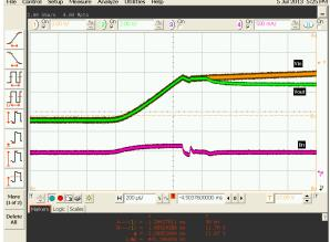
Figure 10 Input Transient Response
