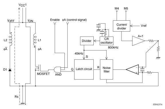
Driver Block Basic Circuit Structure
