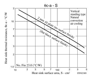
Next we determine the usage conditions with no heat sink by determining the allowable hybrid IC internal average loss from the thermal resistance of the hybrid IC substrate, namely 23°C/W.
