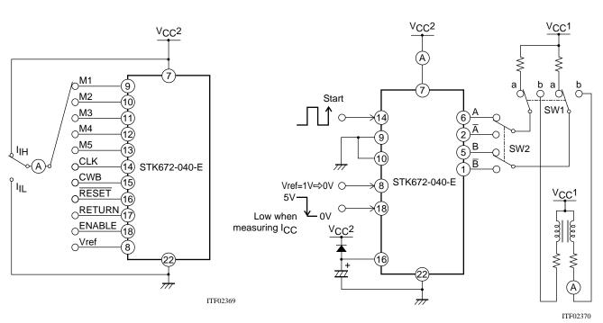
When measuring Ioave: With SW1 set to 'a', Vref = 1V When measuring fc: With SW1 set to 'b', Vref = 0V When measuring ICC: Set ENABLE low
