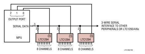
Figure 3. Several LTC1294 Sharing One 3-Wire Serial Interface
