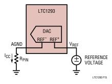
Figure 15. Parasitic Pin Resistance (R<sub>PIN</sub>)
