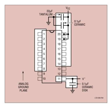
Figure 4. Ground Plane for the LTC1293/4/6
