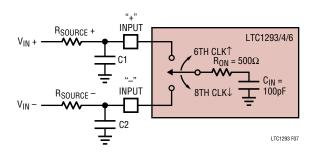
Figure 7. Analog Input Equivalent Circuit
