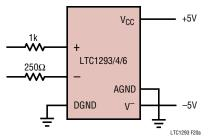
Figure 20a. Overvoltage Protection for Inputs
