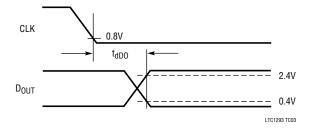
Voltage Waveform for  $D_{OUT}$  Rise and Fall Times,  $t_r, t_f$
