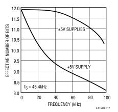
Figure 17. LTC1294 ENOB vs Input Frequency
