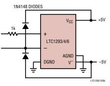
Figure 20b. Overvoltage Protection for Inputs
