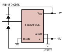
Figure 19. Overvoltage Protection for Inputs
