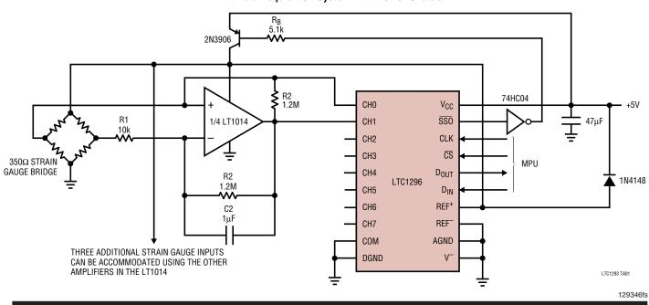
12-Bit Data Acquisition System with Power Shutdown
