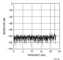
Figure 16b. LTC1294 FFT Plot  $f_{IN}$  = 22kHz,  $f_S$  = 45.4kHz, SNR = 72.5dB with  $\pm 5V$  Supplies
