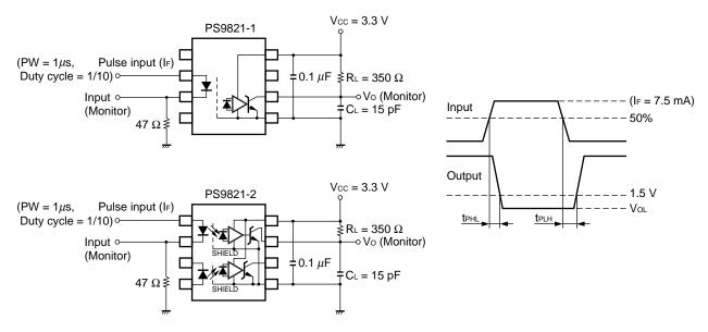
Remark CL includes probe and stray wiring capacitance.
