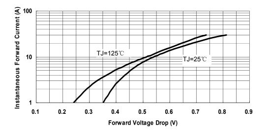
Fig.3-Typical Instantaneous Forward Voltage Characteristics
