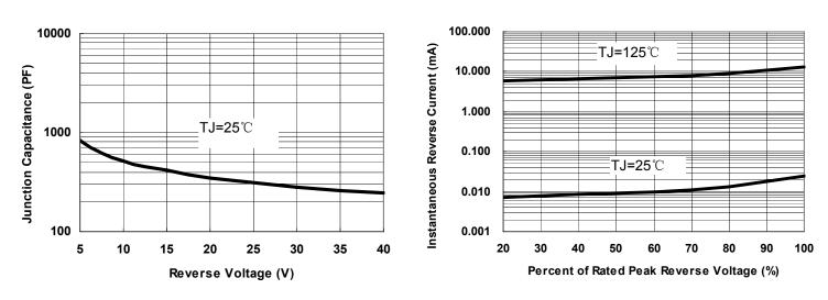
**Fig.1-Typical Junction Capacitance**
