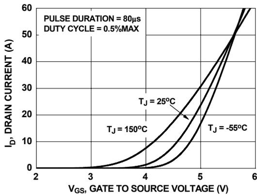
**Figure 5. Transfer Characteristics**
