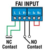
FAI Activates when the NO contact CLOSES. FAI Deactivates when the NO contact OPENS AND the NC contact momentarily OPENS.
