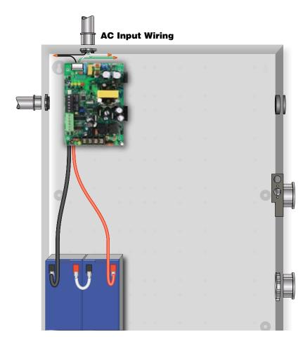
The drawing above shows a typical installation. Actual configuration and wire routing will vary based on the components installed in your system. The following guidelines should be followed for installation.
