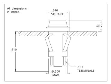
Mounting: Will snap-fit into Ø.500/.505 hole in panels .020/.100 thick. Push-on speednut SN0461 also available.
