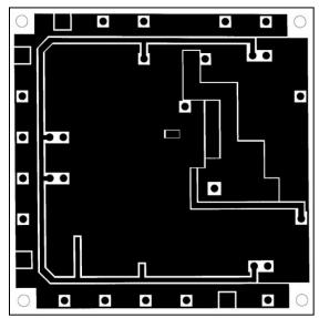
L2 : Copper wiring pattern diagram
