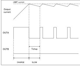
Figure. 4 Waveform of CHOP sequence
