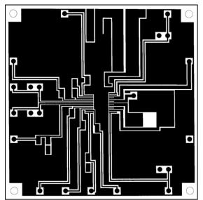
L1 : Copper wiring pattern diagram
