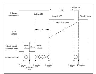
Figure. 6 Waveform of SCP (Latch Mode)
