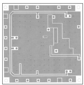
Figure. 11 PCB Design of Solder side.
