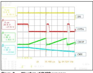
Figure. 9 Waveform of CHOP sequence
