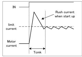
Figure. 5 Waveform of CMK sequence
