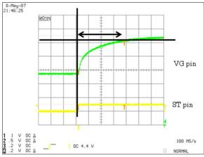
Figure. 3 VM=24V C<sub>VG</sub>=0.1uF Thresh=VM+4V
