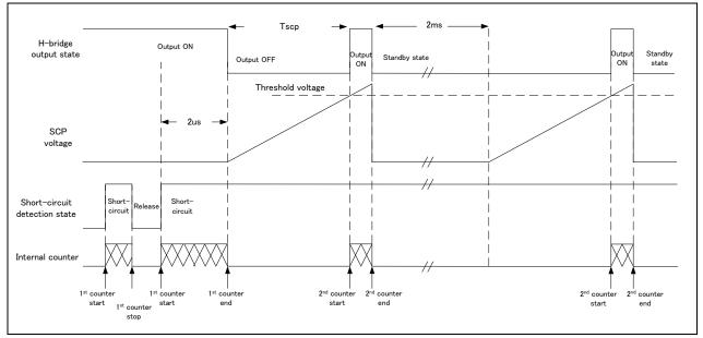
Figure. 7 Waveform of SCP sequence (Auto Retry Mode)
