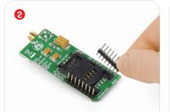
Turn the board upside down so that the bottom side is facing you upwards. Place shorter pins of the header into the appropriate soldering pads.
