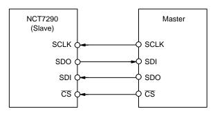
Figure 25. SPI Interface between Master and NCT7290 (Slave)
