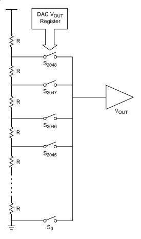
Figure 21. DAC Register String Architecture
