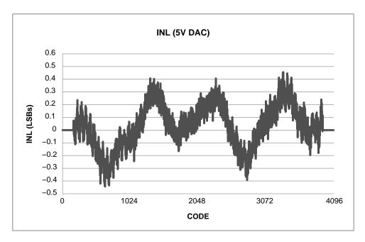
Figure 8. INL vs Code at 25°C for 5 V DAC OUTPUT
