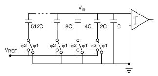
Figure 17. The Conversion Phase of the Typical ADC
