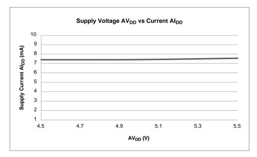
Figure 12. Supply Current vs Supply Voltage
