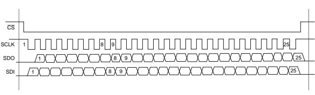
Figure 26. Bit Timing Diagram for SPI Communication
