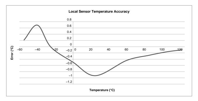
Figure 14. Local Temperature Error vs Temperature
