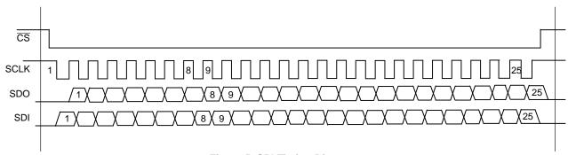
Figure 5. SPI Timing Diagram
