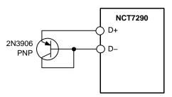
Figure 20. Discrete PNP Transistor as Remote Sensor
