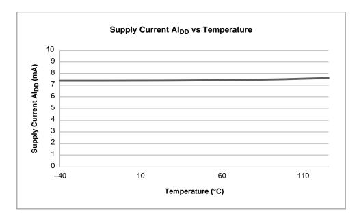
Figure 13. Supply Current vs Temperature
