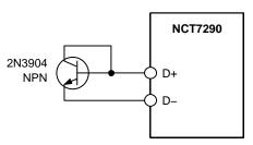
Figure 19. Discrete NPN Transistor as Remote Sensor
