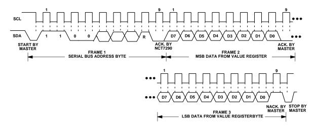
Figure 23. Reading a Word from a Previously Selected Register
