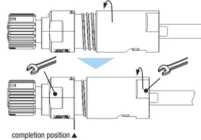
\*2 When screwing up the cap by large size tool, it may cause damage.
