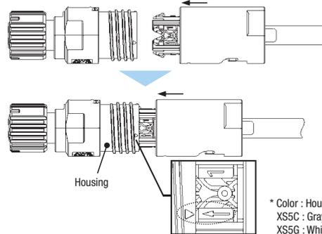
\* Confirm that the color of the housing and the IDC cover is same before insertion.
