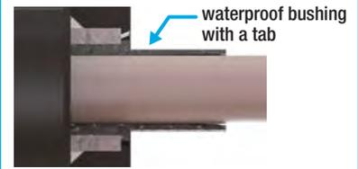
Handles cable diameters of 3 to 8 mm. For 5 to 8-mm dia., just remove the tabbed, waterproof bushing.
