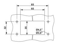
Panel cutout  $\,^{2)}$  When self-tapping screws are used (Torx® 20, M4)
