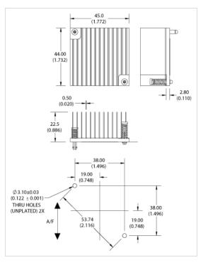
Width: 45.00 Length: 44.00 Height: 22.50 Base Thickness: 2.80 Fin Thickness: Length , Width 0.50 # of Fins: Length , Width 13 Fin Tip to Tip: Finish: AavSHIELD 3C
