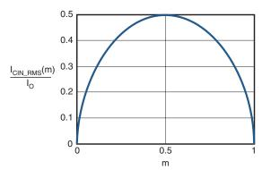
Figure 2. I<sub>CIN</sub> vs. Voltage Conversion Ratio
