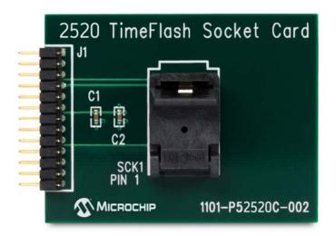
Single socket card, 2.5 x 2.0 mm, with 10 blank DSC8001 parts for TimeFlash Oscillator Programming Kit
