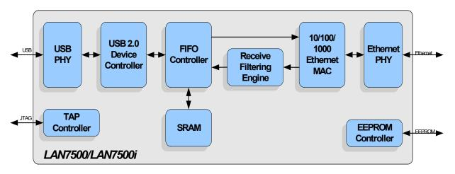
Figure 1 LAN7500/LAN7500i System Diagram
