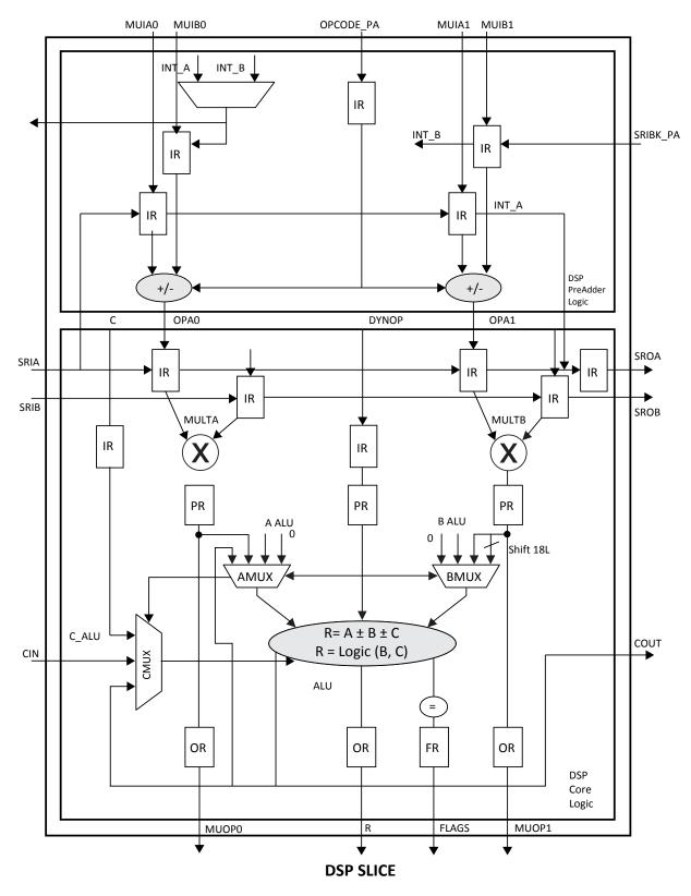
Figure 2.15. Detailed sysDSP Slice Diagram
