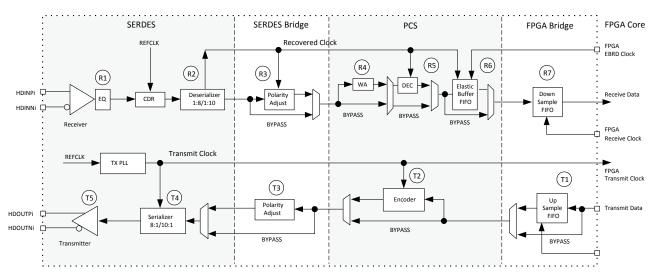
Figure 3.13. Transmitter and Receiver Latency Block Diagram
