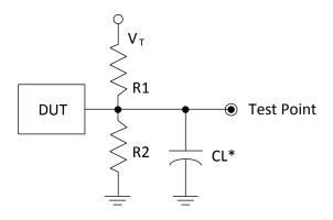
\*CL Includes Test Fixture and Probe Capacitance
