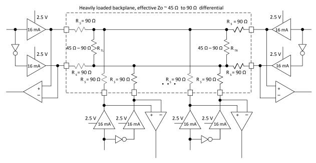
Figure 3.2. BLVDS25 Multi-point Output Example
