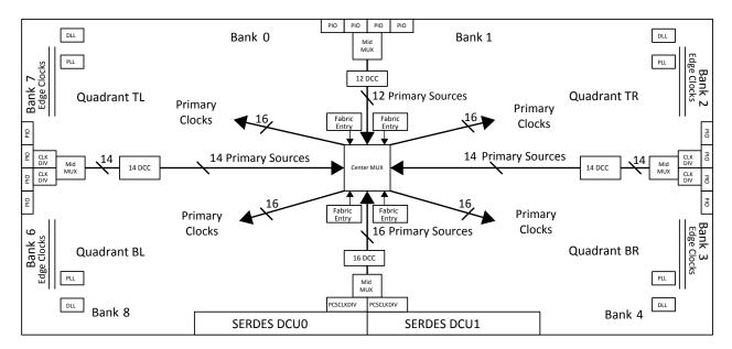
Figure 2.6. LFE5UM/LFE5UM5G-85 Clocking
