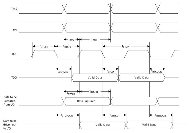
Figure 3.23. JTAG Port Timing Waveforms
