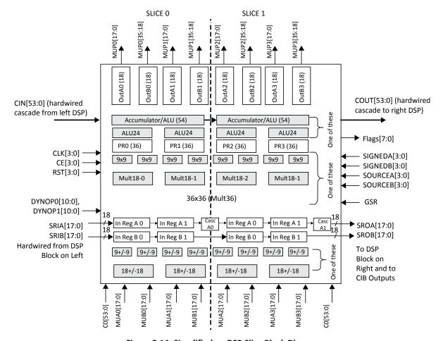
Figure 2.14. Simplified sysDSP Slice Block Diagram
