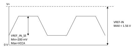
Figure 3.14. SERDES External Reference Clock Waveforms
