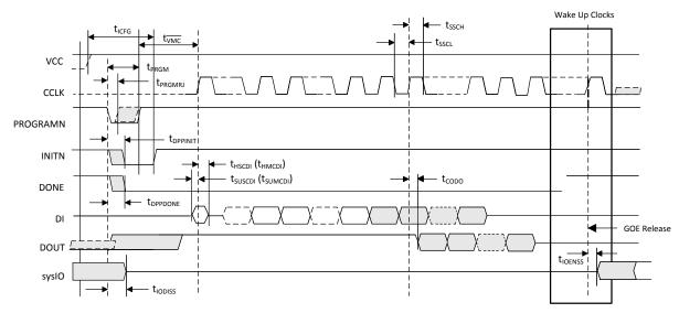
Figure 3.19. sysCONFIG Port Timing
