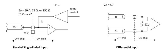
Figure 2.26. On-Chip Termination
