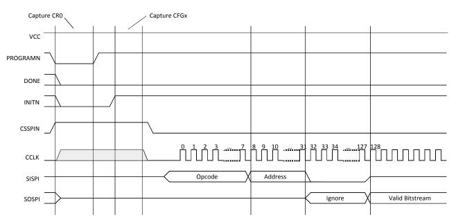
Figure 3.22. Master SPI Configuration Waveforms
