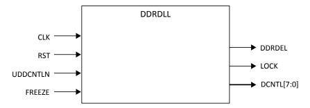
Figure 2.10. DDRDLL Functional Diagram
