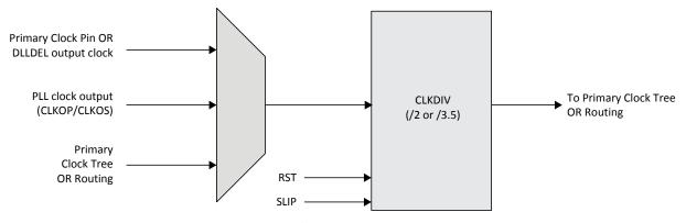
Figure 2.9. ECP5/ECP5-5G Clock Divider Sources
