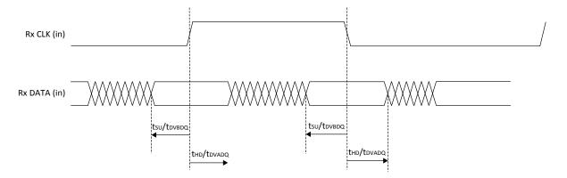
Figure 3.6. Receiver RX.CLK.Centered Waveforms
