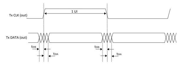
Figure 3.9. Transmit TX.CLK.Aligned Waveforms
