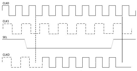
Figure 2.7. DCS Waveforms
