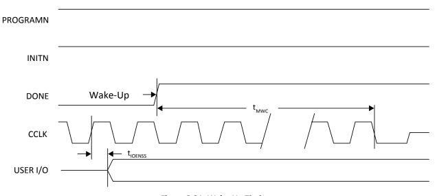
Figure 3.21. Wake-Up Timing
