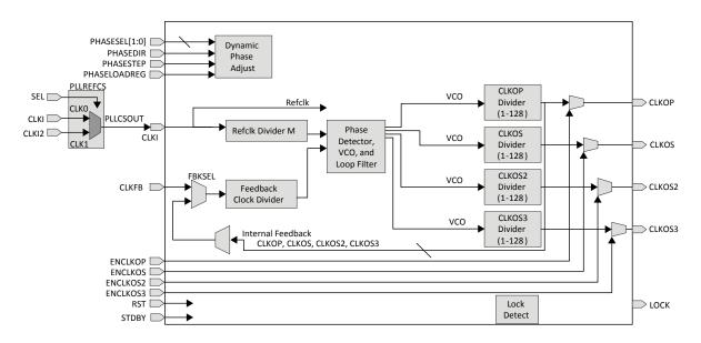
Figure 2.5. General Purpose PLL Diagram
