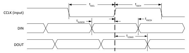
Figure 3.17. sysCONFIG Slave Serial Port Timing
