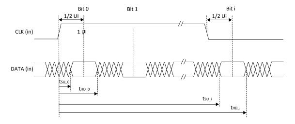
Figure 3.11. Receiver DDRX71\_RX Waveforms
