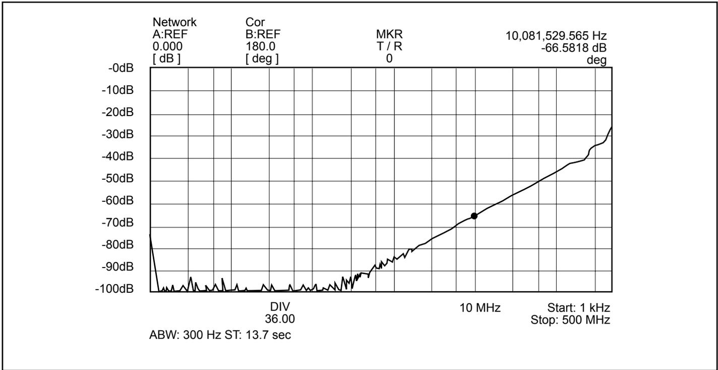
**Crosstalk** ( $V_{CC} = 3.3V, 25^{\circ}C$ )
