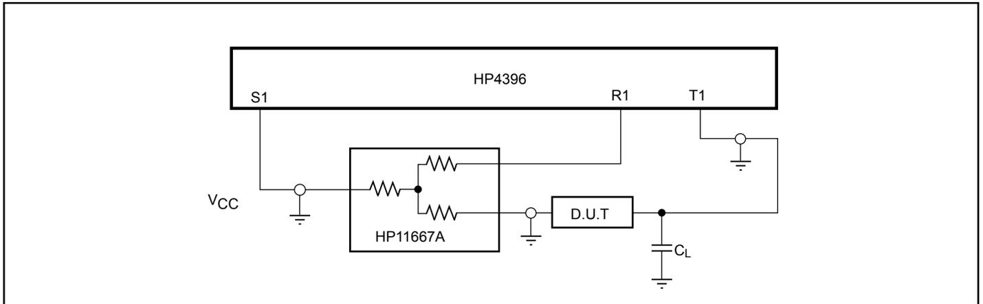
**Off Isolation** ( $V_{CC} = 3.3V, 25^{\circ}C$ )
