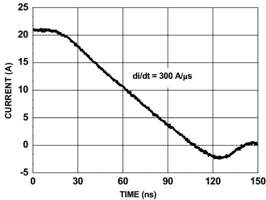
Figure 14. FDMS7670AS SyncFET body diode reverse recovery characteristic
