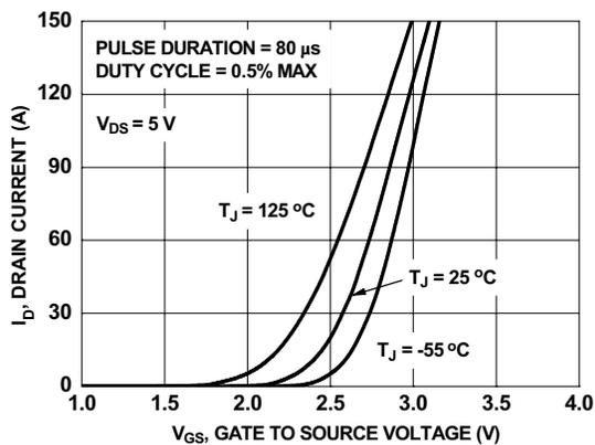
**Figure 5. Transfer Characteristics**
