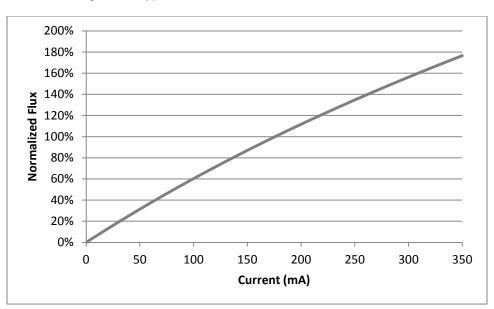
Figure 4: Typical Flux vs. Current - BXRE-xxx-0800-A-xx
