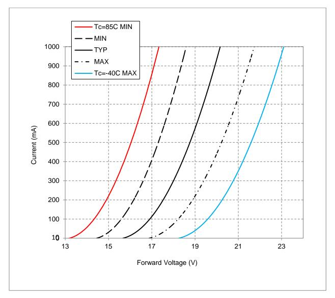
Figure 3: Typical Current vs. Voltage – BXRE-xxx0800-B-xx
