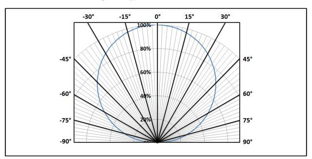
Figure 10: Typical Polar Radiation Pattern
