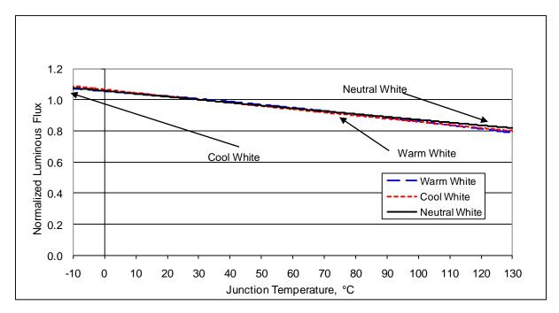
Figure 6: Typical Flux vs. Junction Temperature
