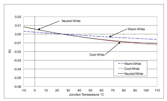
Figure 7: Typical ccy Shift vs. Junction Temperature
