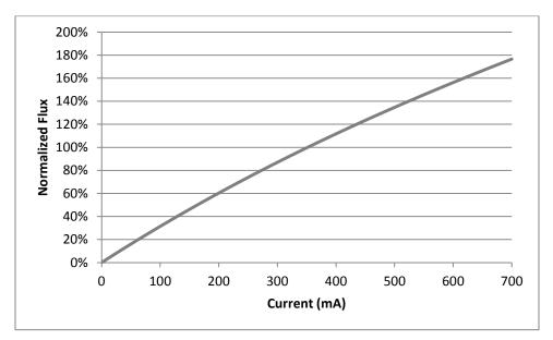
Note: Bridgelux does not recommend driving high power LED Arrays at low currents. Doing so may produce unpredictable results. Pulse width modulation (PWM) is recommended for dimming effects.
