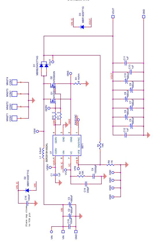
Figure 7. NCV8871BSTGEVB Evaluation Board Schematic
