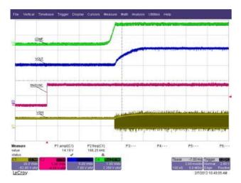
Figure 6. Soft Start with Load
